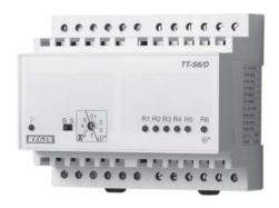
TT-S6/D is a microprocessor based step controller for controlling electric heaters etc. The step controller is controlled by a 0...10V signal from a TTC25/TTC40F regulator or from another controller or DDC.
