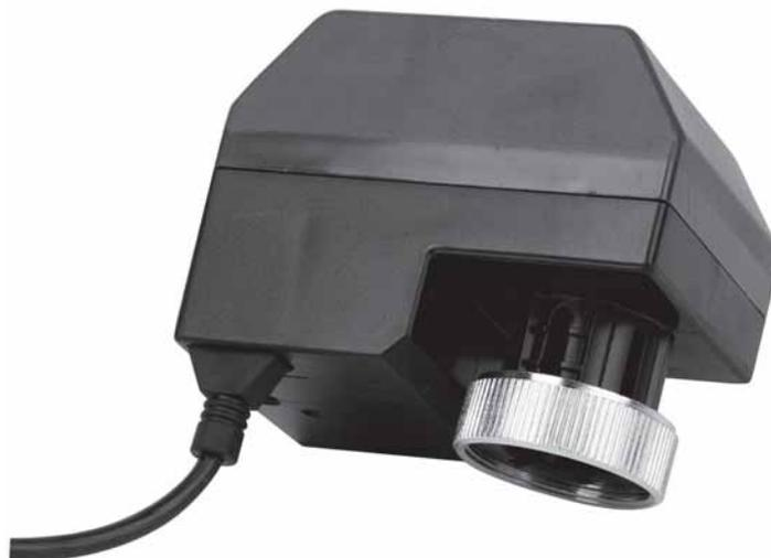
MVT44 / MVT57 are valve actuators for three point floating or 0...10 V control signals. The actuators are intended for use together with valves in the VST / VMT series.
