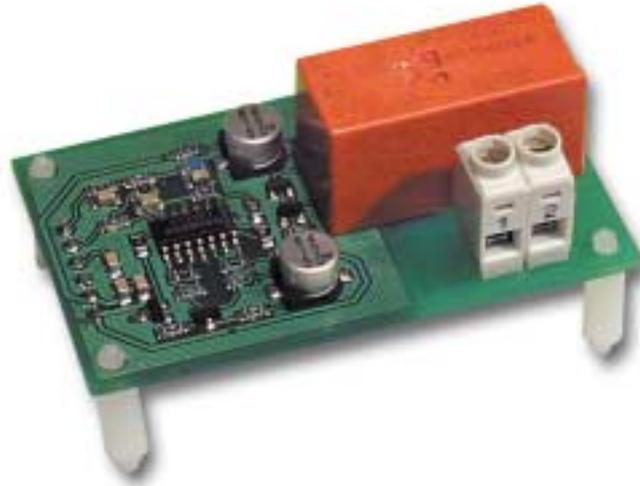
**TT-S1 is an ancillary board intended to control extra load when using the TTC2000 controller.**
