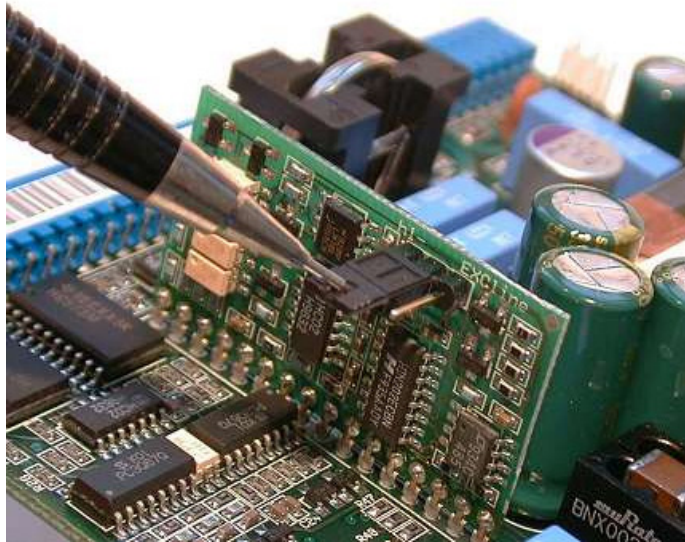
Figure 68. The jumper for selecting EXOline/hlEXOline.
